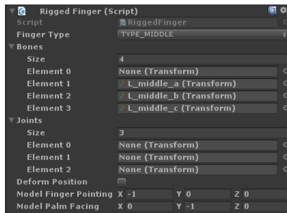
Figure 5. Character rigging is performed for each segment of the arm . Fig 5. represents the character rigging performed for a single finger in the arm.
