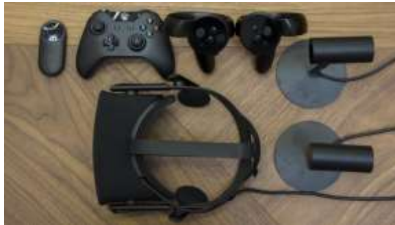
Figure 9. The above figure shows the complete oculus rift setup with the headset , IR sensors ,controllers, remote and joystick.
